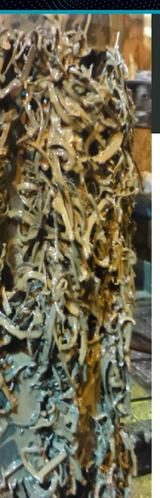
In some situations casing milling prior to cement placement is required to achiveve an effective cement-to-formation seal during wellbore abandonment.
